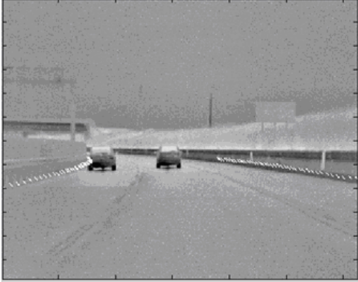
Fig. 5 Road borders tracking projected in image plane
